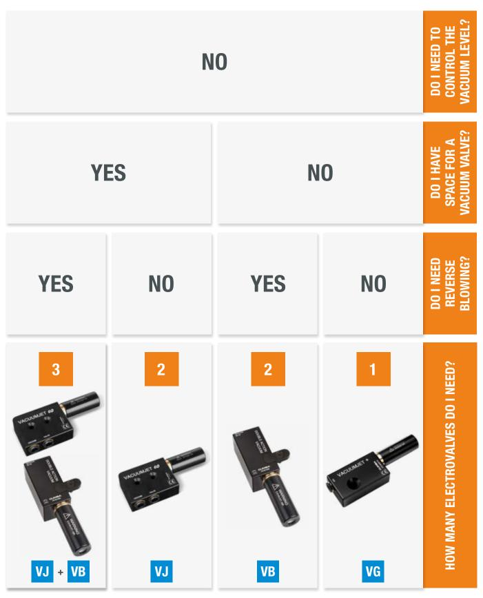
The use of Spiral Ejector or Spiral Sleeve (VP & VS) is mandatory when not using a valve. However, it is also recommended when using a valve to maintain the vacuum achieved throughout the rest of the process.
